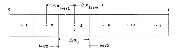
Figure 4.5 Block-Center Grid in Finite-Difference Approximation.
