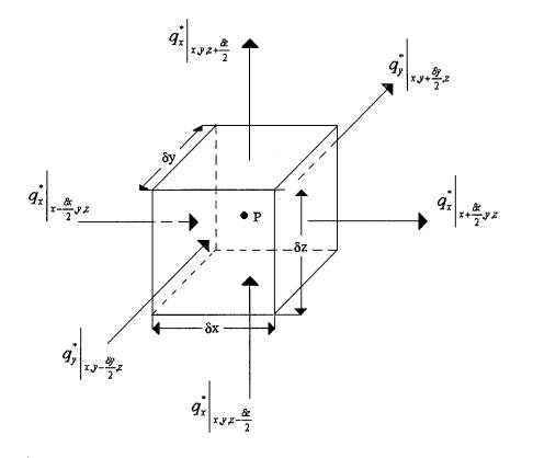
Figure 4.2 Schematic Diagram Showing the REV and the Fluxes q\*.
